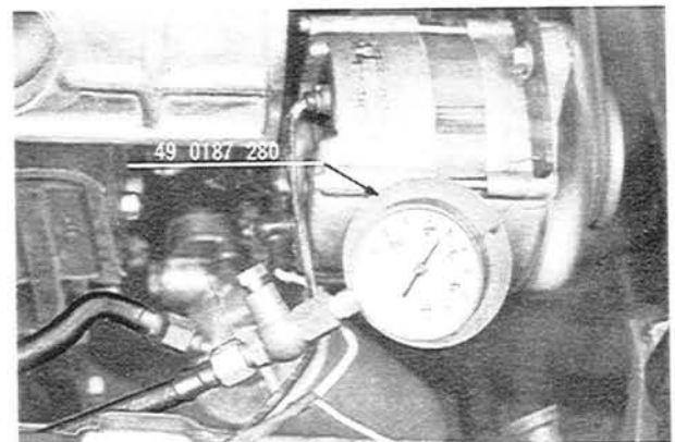
Fig. 2-3 Checking of oil pressure.
